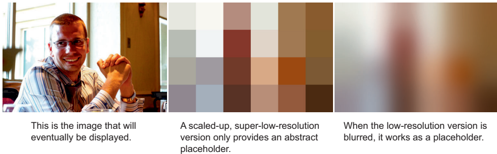
Figure 8.12 Using a blurred version of a low-resolution copy of an image makes an excellent placeholder until the final image can be displayed.
