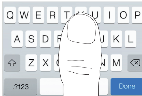
Figure 5.1 It's hard to tell what key is being pressed when a finger (or thumb) covers multiple targets.
