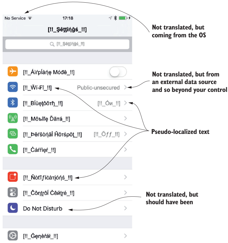
Figure 3.2 An app configured to use a pseudo-loc translation makes it easy to spot any words that aren't coming from a correctly translated language resource.
